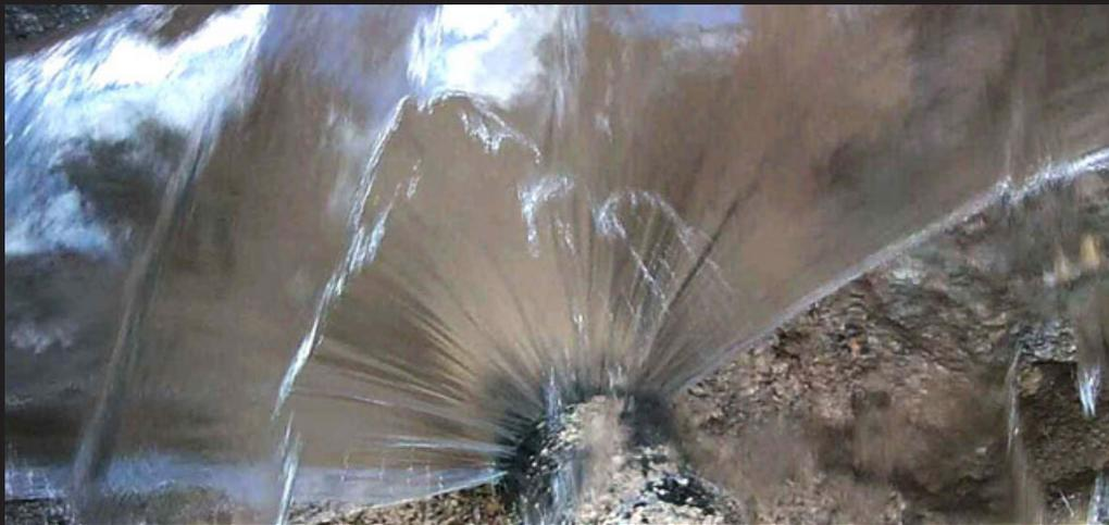
To locate leaks, look for any trend of increased usage that cannot be associated with increased business through sub-meters.
