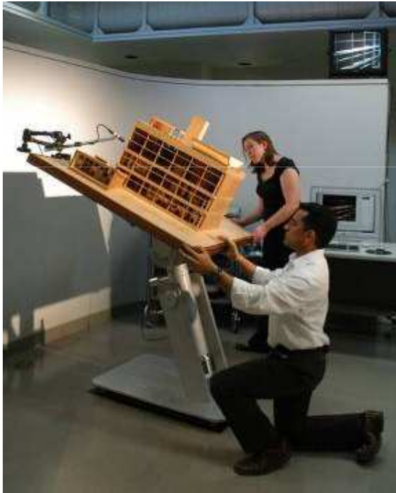
Analysis of an architectural model using the heliodon, which simulates sunlight penetration and shading at different times of day and during different seasons
